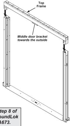
At this point, resume the assembly procedure at Step 8 of "Floor Frame and Door Frame Assembly" in the SoundLok Sound-Isolation Room Assembly Instructions 270A673.
